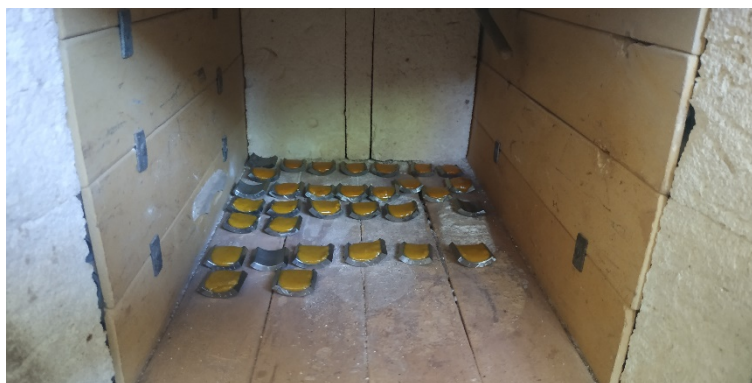
Figure 1. Samples of steel with the synthetic ash mixture inside the muffle
